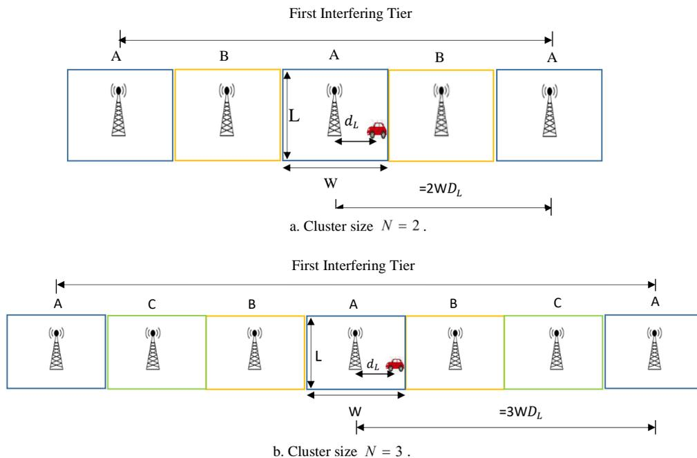
Fig. 2. The linear system with rectangular shape.
