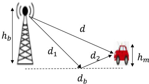
Fig. 4. Physical arrangement of dual-slop propagation.
