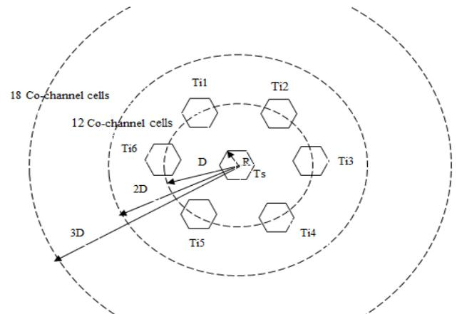
Fig.1. Interfering cells in a hexagonal arrangement [15].
