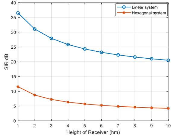
Fig. 11. Effect of Mobile height  $h_m$  on SIR.
