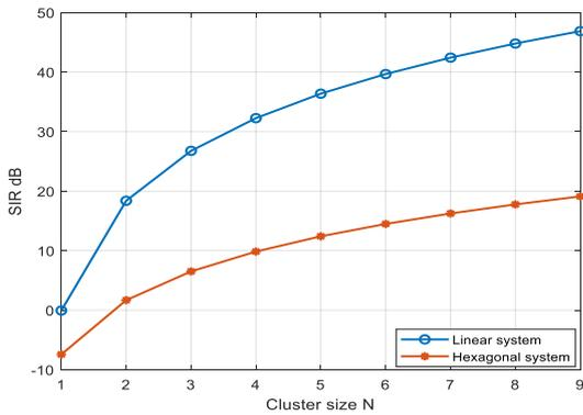
Fig. 7. Effect of Cluster Size on SIR in log-distance model.
