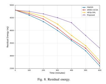
residual energy. Energy performance is critical in disaster networks where recharging or replacing devices is infeasible. The proposed system maintains a high energy efficiency of 0.98 Mbit/J and a residual energy of 4778 mJ, even under increased node activity. This improvement stems from APRO's cost-aware routing, which balances the load, minimizes retransmissions, and avoids energy-depleting paths. In com-
