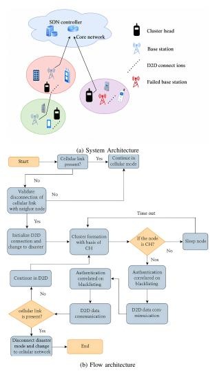
Fig. 1. (a) System architecture and (b) Flow Architecture
