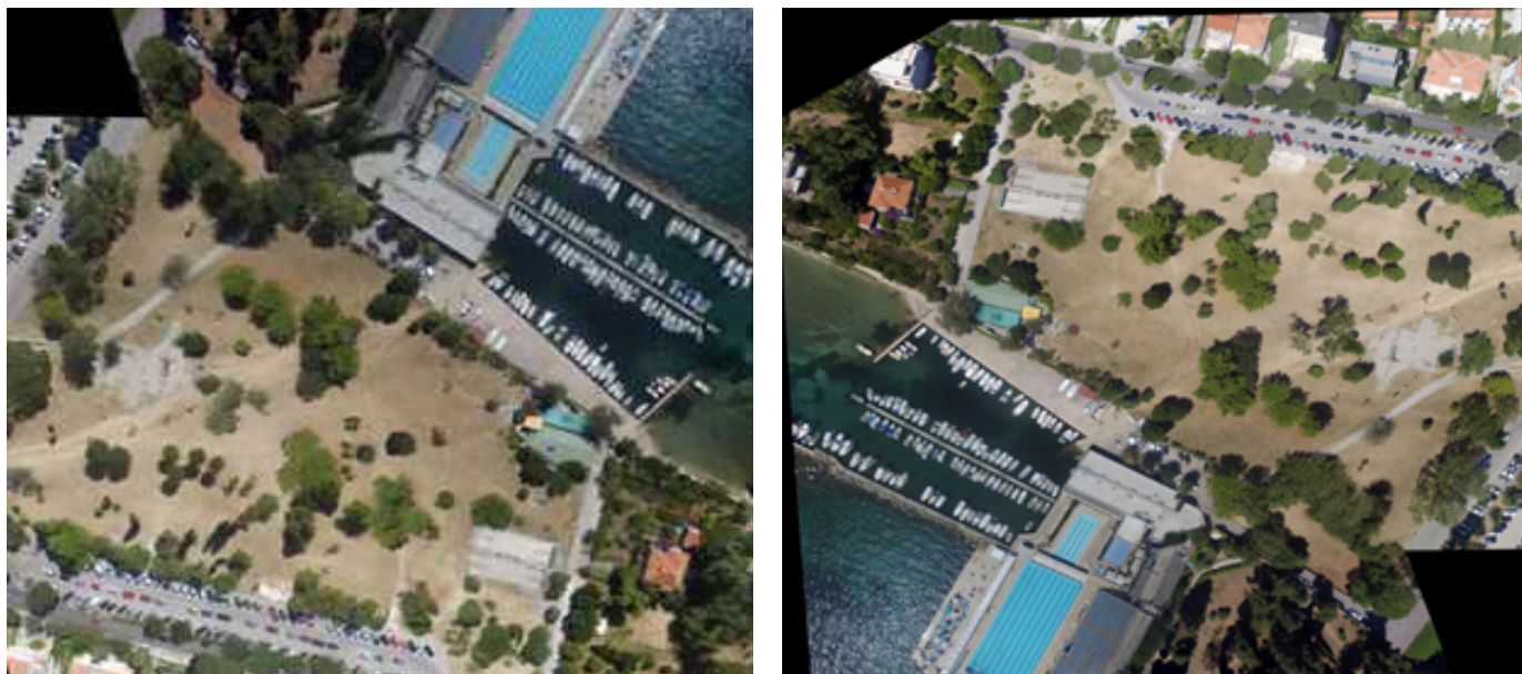
Fig. 3. Image mosaic of the area of interest before (left) and after (right) applying world file transformation
