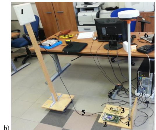
Fig. 2. a) Architecture of the proposed RFID tag characterization system. b) Measurement setup: 1. Reader antenna, 2. Reader board 3. Driver Board, 4. Stepper Motor, 5. Coax Cable.
